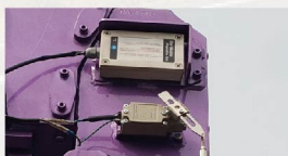
Overwinding Prevention System
